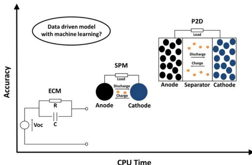
Figure 2. Accuracy vs. CPU time for equivalent circuit model (ECM), single-particle model (SPM) and pseudo 2D model (P2D). Data-driven model (DDM) with machine learning is a new type of battery model that is promising for fast and accurate battery state predictions.
