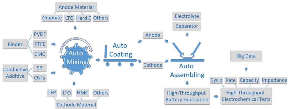
Figure 3. High-throughput battery fabrication and testing. Abbreviations: PVDF: polyvinylidene fluoride, PTFE: polytetrafluoroethylene, CMC: carboxymethyl cellulose, SP: Super P, CNTs: carbon nanotubes, LTO: lithium titanate, Hard C: hard carbon, LFP: lithium iron phosphate, LCO: lithium cobalt oxide, NMC: lithium nickel manganese cobalt oxide.
